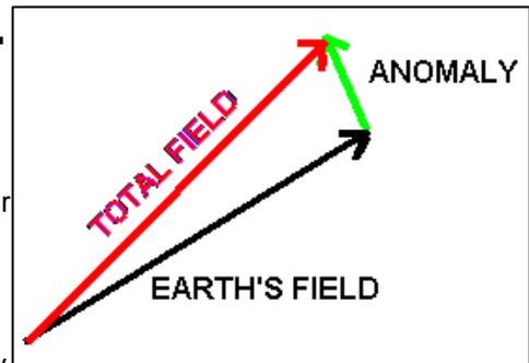
Keep in mind that this vector addition is happening in three dimensions. The computed azimuth of the tool is relative to the **horizontal** component of the **total** field.
